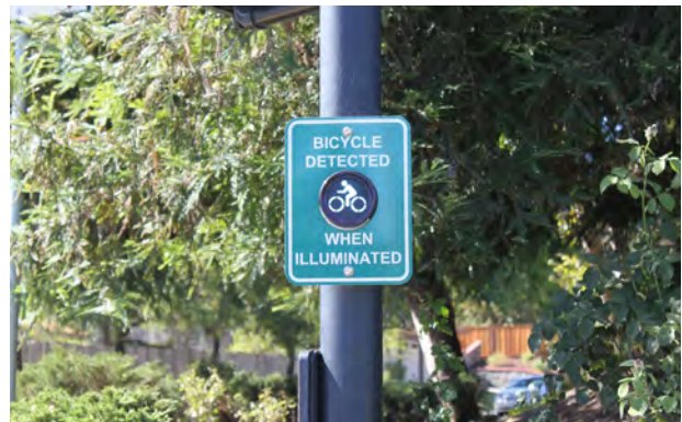
Passive bicycle detection and signage. Passive detection is most often accomplished through video cameras or induction loops.
