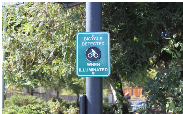
Passive bicycle detection and signage. Passive detection is most often accomplished through video cameras or induction loops.
