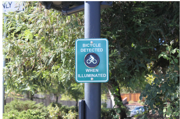
Passive bicycle detection and signage. Passive detection is most often accomplished through video cameras or induction loops.
